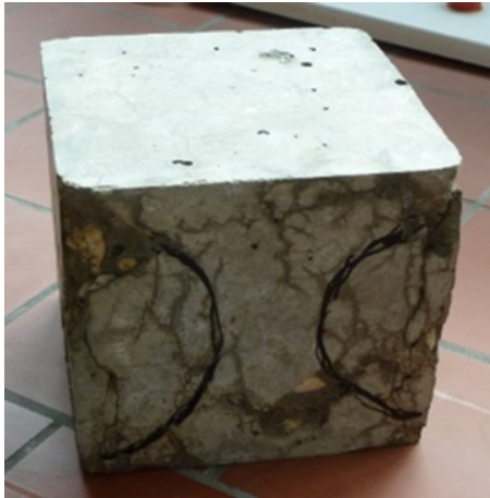
Fig. 38 Fracture paths in a concrete sample cube
