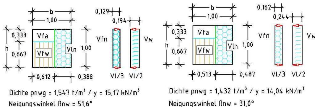
Fig. 65 shows the 'soil band' of the wet sand under water
