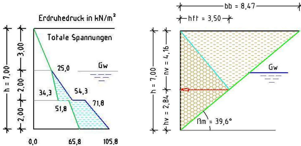
Fig. 67 shows the stresses of the soil under water according to the current teachings, whereby the number values are claimed to correspond to the total stresses.
