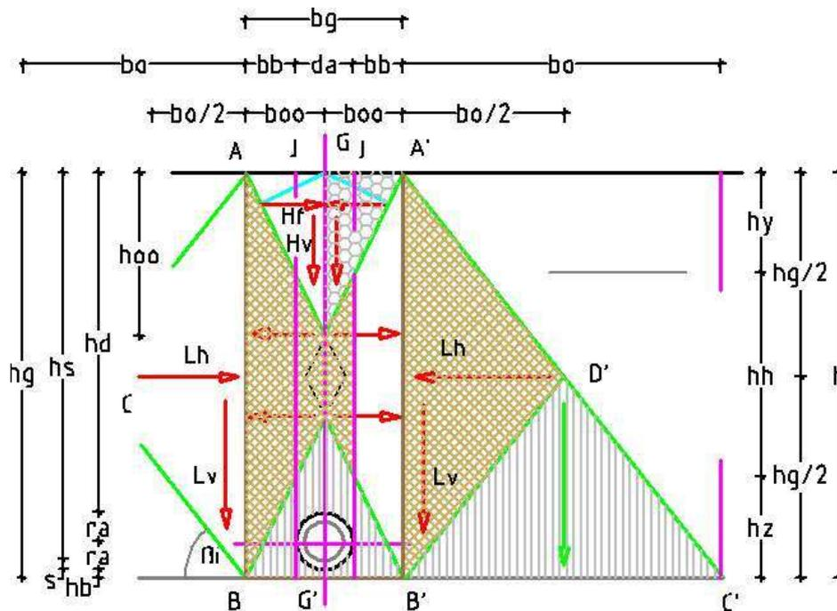
Fig. 56 shows the earth wedges of the trench backfilling at center, and those of the adjacent soil at left.
