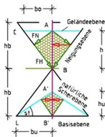
Fig. 1 shows unequal soil bodies and earth forces in an hourglass.
