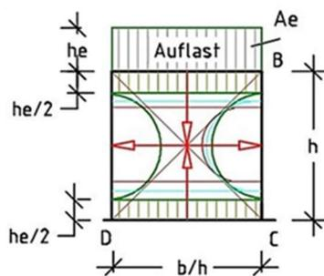
Fig. 39 only shows symmetrical fracture and force paths in the cube.
