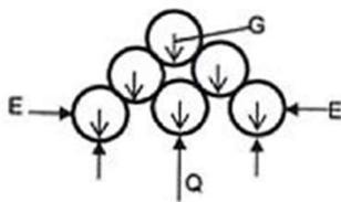
Pict. P02.20 shows that in a heap of spheres with horizontal support, force dispersal is only possible in the vertical direction.
