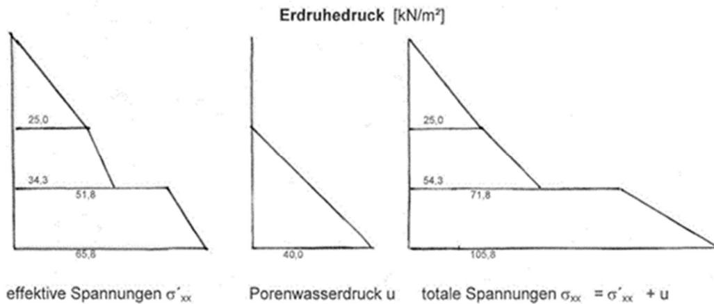
Bild L-4: Substratum and stress determination of the Center for Geotechnics at the TUM
