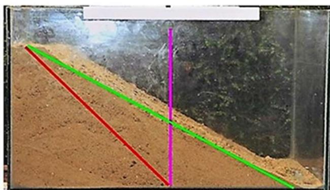
Fig. 22 shows the inclination plane (red) and the shear plane (green).
