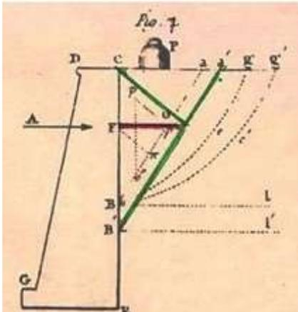
The division of area  $(a-a'-B'-B)$  forms a steeper inclination angle  $\beta_e$  and lengthens the friction/inclined plane.
