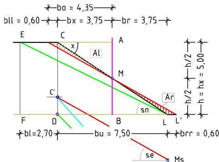
Fig. 61 shows the embankment plane (C-L), shear plane of moist soil (E-L), and shear plane of wet soil (C'-H').
