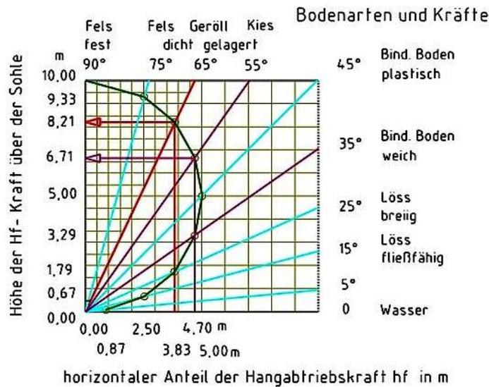
Fig. 11 shows the dependencies of inclination angles and earth pressure forces, and their thrust heights against the wall in the 'semicircle of soil type'.
