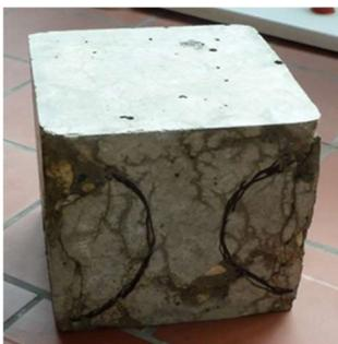
Fig. 38 shows the fracture paths in the concrete test cube.
