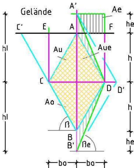
Fig. 52 shows the force areas at left without live load, and at right with live or static load.
