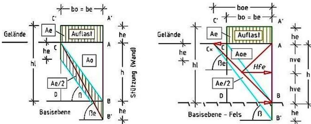
Fig. 36 shows the inclined planes without/with load and vertical force dispersal.
