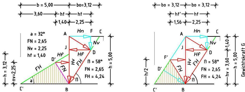
Fig. 9 shows lying earth wedge at left of axis A-B, and the standing earth wedge at right.
