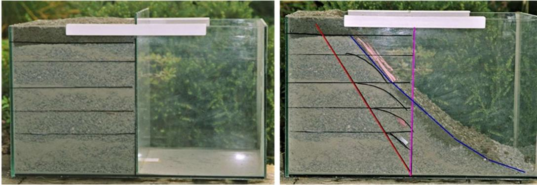
Fig. 28 shows the basalt grit layers in the left chamber of the glass container.
