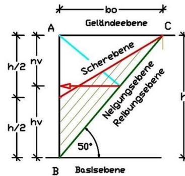
Fig. 23 shows an earth wedge standing on its point with inclination angle  $\beta$ .
