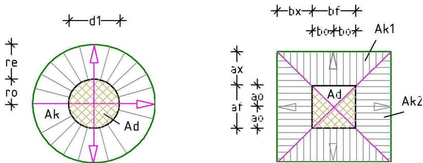
Fig. 20 shows a circular foundation with radial force dispersal over area  $A_k$ .
