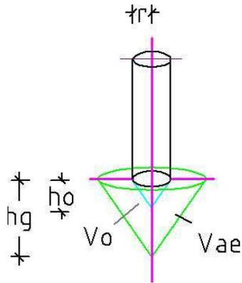
Fig. 49 shows force dispersal of the load and of the soil's own weight.
