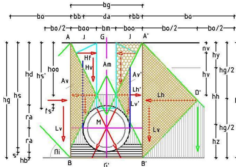
Fig. 58 shows the pipe, embedded in the force areas of the rhombus acc. to Figs. 53 and 54.
