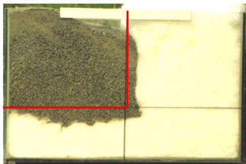
Fig. 55 shows the displacement of the lighter soil by the heavier trench backfilling.
