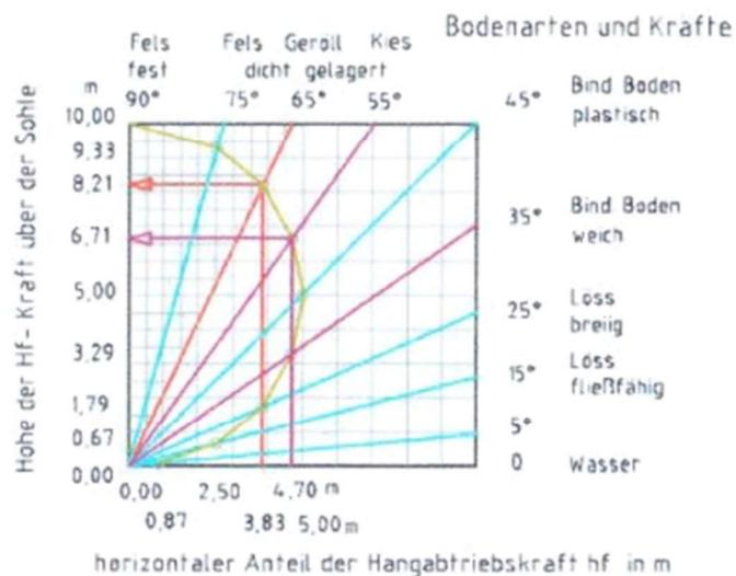
**Fig. 11** shows the 'Semicircle of soil types' with the dependencies on inclination angle, earth pressure force, and their thrust heights against a wall.
