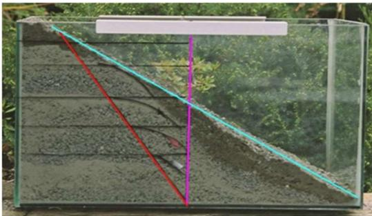
Fig. 30 shows the newly formed linear shear plane of the grit after removal of the upper paper strip.
