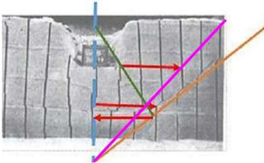
The visible traces in the sand show a dispersal of the pressure force in the horizontal direction, and the formation of new friction planes under angle  $\beta_e$ .
