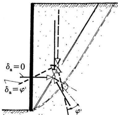
1. On the rear side of a rough wall, thrust forces occur which can influence earth pressure inclination angle  $\delta_a$  and earth pressure force  $E_a$ .
