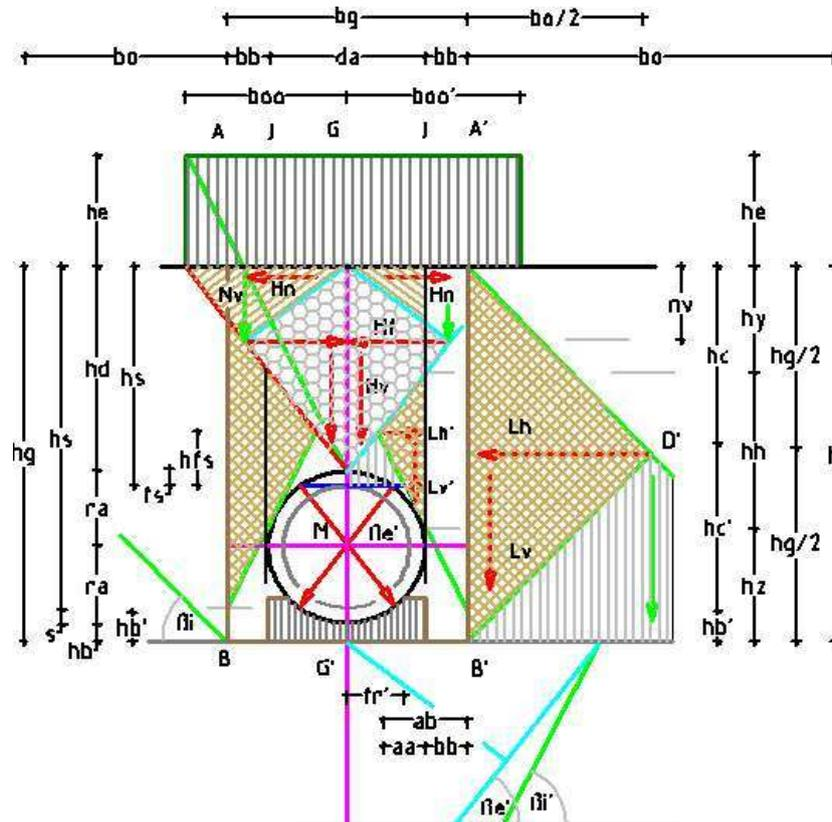
Fig. 59 shows the drain pipe bedded in concrete, and its force areas.
