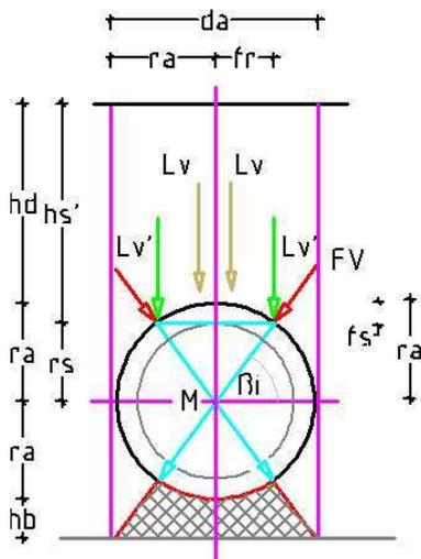
Fig. 57 shows the force distribution on the drain pipe.
