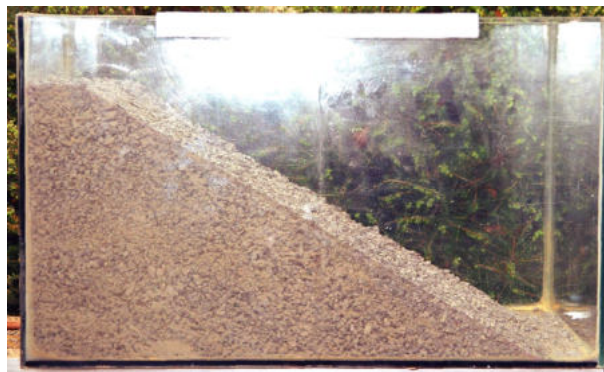
Fig. 43: Position of shear plane of the moist basalt grit.
