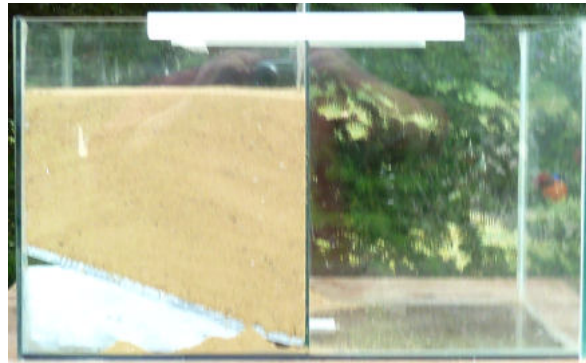
Fig. 96: Glass container with built-in wooden ramp, whose surface represents an inclined rock layer.
