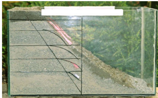
Fig. 30 Basalt grit and paper strips after removing the separating glass pane.
