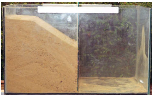
Fig. 76: Sand body with partially inclined surface.
