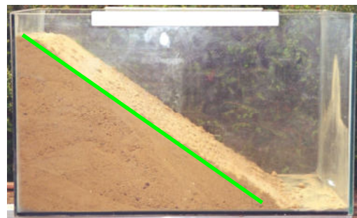
Fig. 77: Shear plane after the sand has slipped down.
