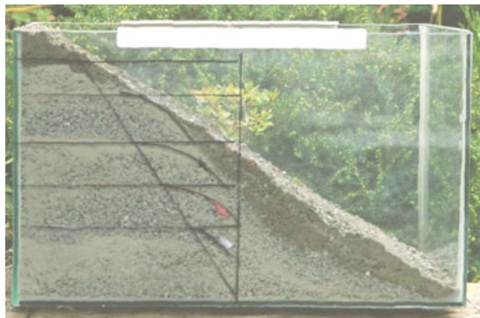
Fig. 31 Basalt grit after pulling out the paper strips from the two upper layers.
