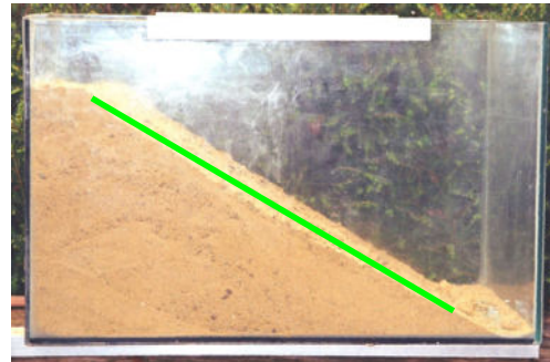
Fig. 74: Shear plane (green) and the sand's shear angle s .
