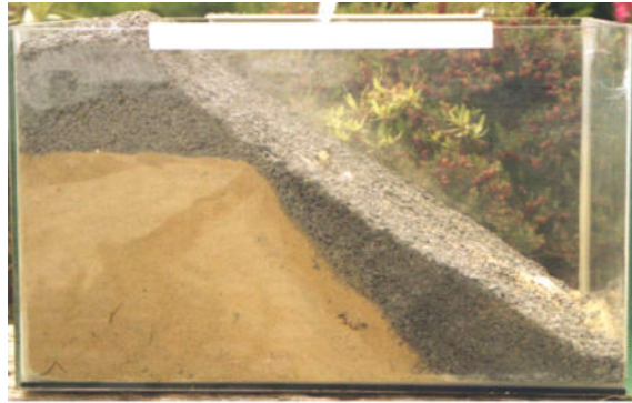
Fig. 32 Inclination plane of the sand, and shear plane of the grit after the filling material had slipped down.
